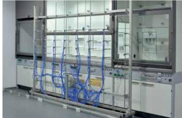
EN 14175-6 type tested fume hood control in acc. with 5.4
