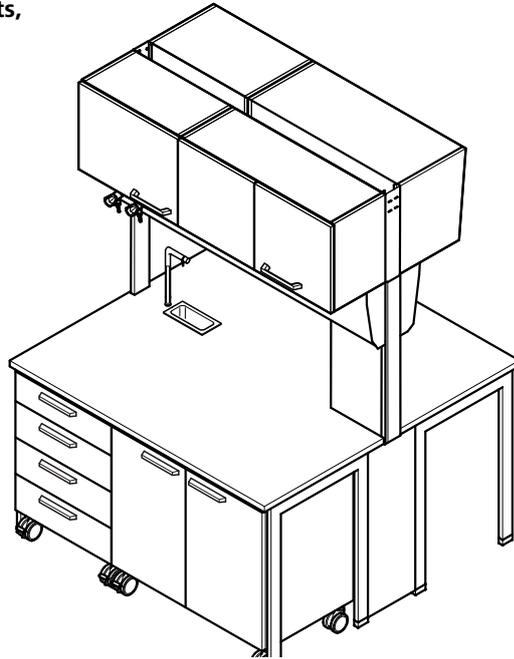
Bench-mounted service duct with overbench cabinets, pillar extension and underbench units on plinth
