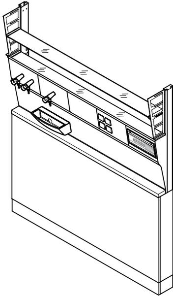
Service spine for wall bench with C-frame, underbench units on castors and overbench cabinet, working height 750 mm
