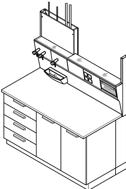
Service spine for double bench with underbench units on plinth and media supply from above, working height
