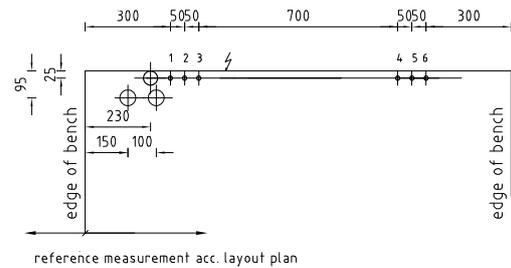
reference axis = finished wall (wall working bench)
