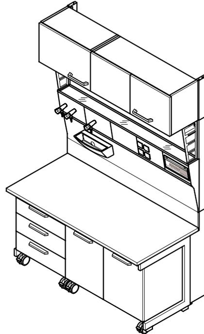
Service spine for wall bench with underbench units on plinth and media supply from above, working height 900 mm
